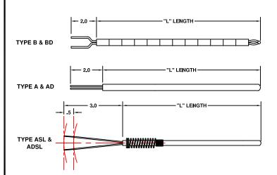
ELEMENT "L" LENGTH EQUALS ASSEMBLY "U" + "F" + "A" + HEAD EXTENSION ADDER BELOW.
