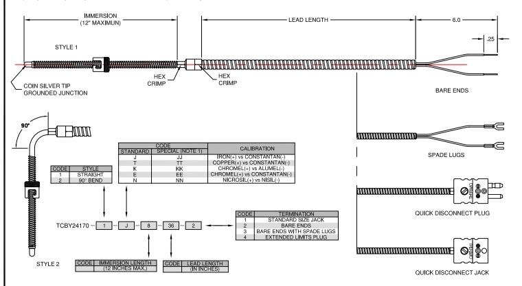
This variable depth thermocouple adjusts to any immersion length. The locking cap rotates on the ridges of the flexible Stainless Steel armor tubing. The probe remains in constant contact to the measured surface by the compression of the armor assuring rapid heat transfer to the thermocouple measuring junction.
