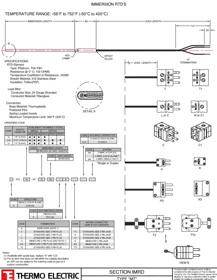
IMMERSION RTD'S with LEAD WIRE SINGLE & DUPLEX CONSTRUCTION outside the recipients organization without the written permission of Thermo Electric.
